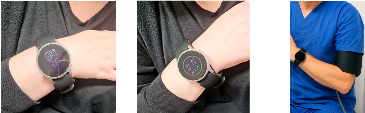
Figure 1. Measurement with Omron HeartGuide: The device is positioned at heart level in accordance to the instructions on the display (left); after the measurement, blood pressure values are displayed (middle); photograph with both devices, the Omron HeartGuide (worn on the wrist) and the ambulatory blood pressure (worn on the upper arm) (right).
