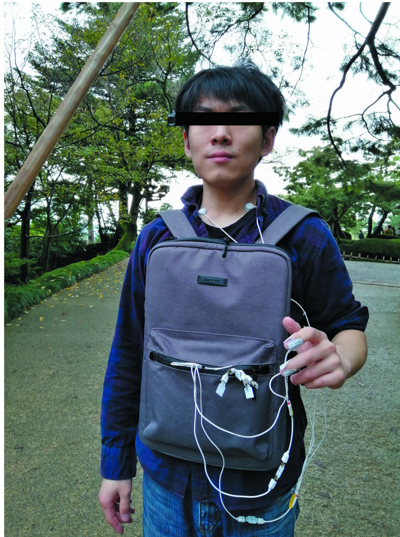
Fig 4. The participants wore a physiological signal feedback device (BITalino (r)evolution Plugged kit), carried a GPS device (Nav-u NV-U73T, Sony) and a laptop computer as they walked through the selected space route at a natural pace and constant speed. They could turn their heads to look at their surroundings. The computer automatically recorded the EDA, ECG, and EMG. The position where the electrodes of the physiological signal feedback instrument were pasted on the body: the two EDA electrodes were fixed on the first phalanx of the index and middle fingers; the ECG electrodes were fixed at the carotid arteries on both sides of the neck; the EMG electrodes were fixed on the inner side of the forearm of the arm.
