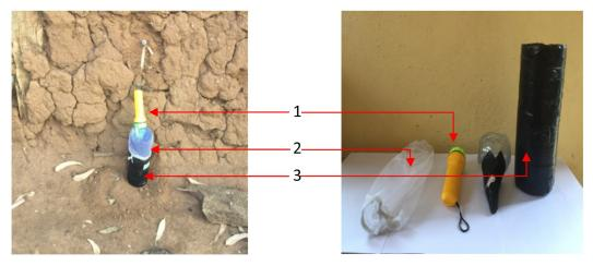
Fig 2. The handmade trap evaluated in the field: (1) torch suspended at 5 centimeters above the trap entrance, (2) gauze net, (3) a <sup>3</sup>/<sub>4</sub> cut plastic bottle wrapped with black scotch tape.
