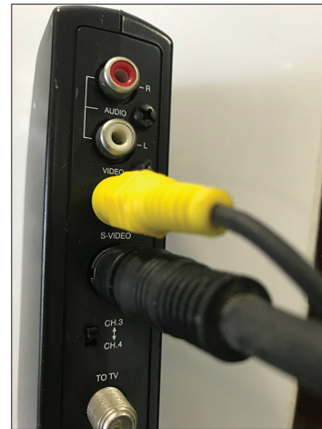
Figure 5: Radio frequency modulator converting an S-video to composite video
