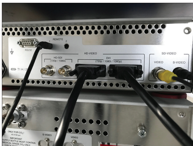
Figure 3: Three-chip camera system showing standard definition and high-definition connections
