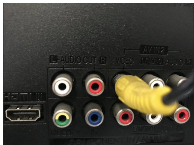
Figure 4: Radio Corporation of America plug connected to the television monitor
