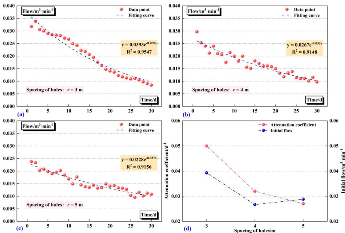
Figure 11. Characteristic curves of average drainage amount, drainage attenuation coefficient, and initial drainage amount under different spacings of hole arrangement; (a–c) characteristic curves of average drainage amount of a single hole; and (d) characteristic curves of drainage attenuation coefficient and initial drainage amount.
