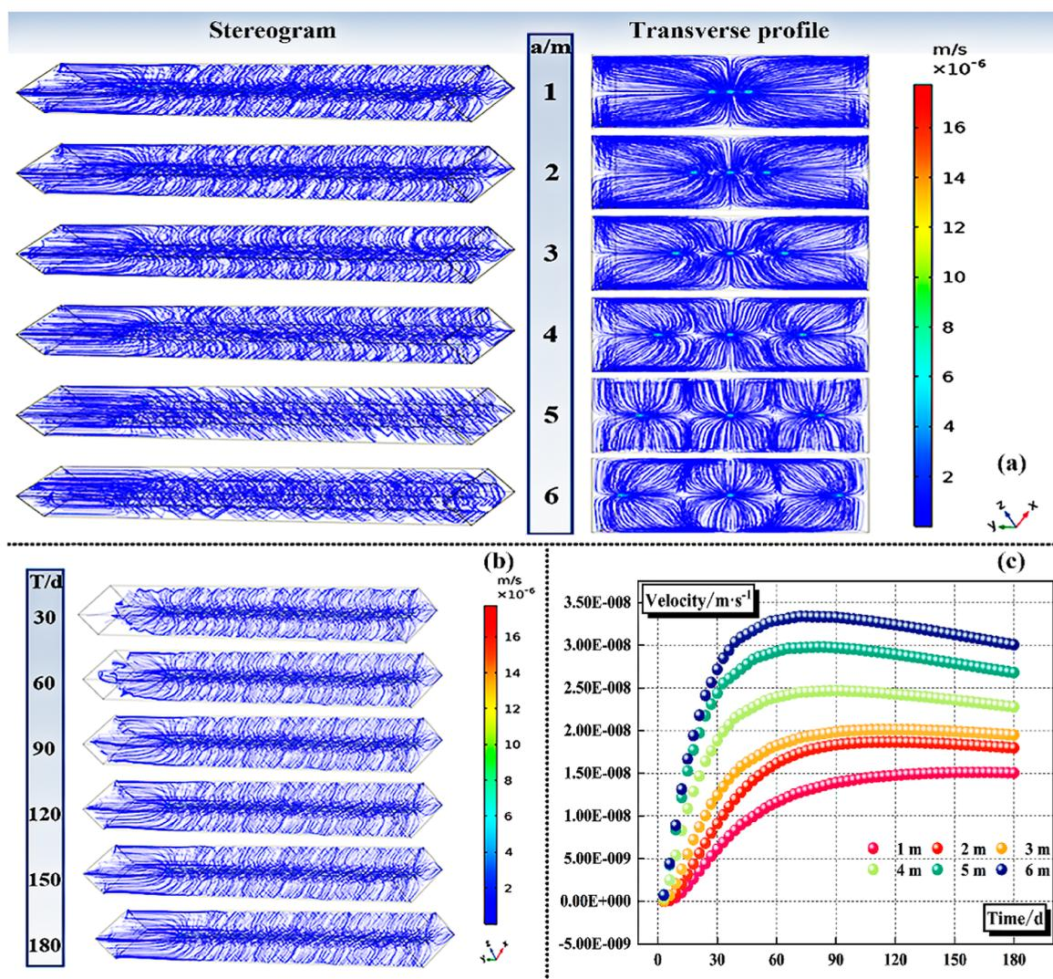
**Figure 5.** Gas migration velocity field distribution results; (a) velocity field distribution with different borehole layout spacings; (b) velocity field distribution over time with 1 m borehole layout spacing; and (c) velocity volume change at the node.
