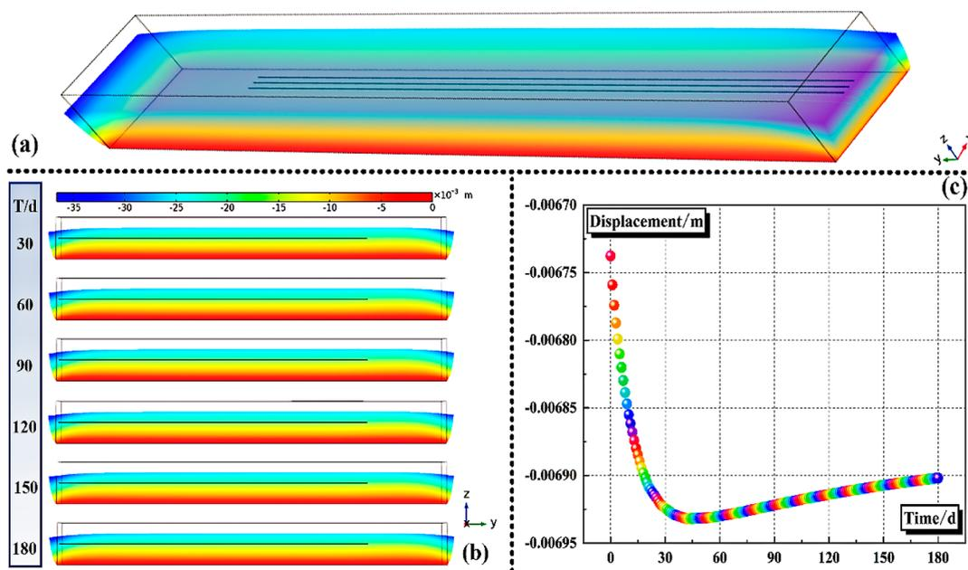
Figure 4. Z-direction displacement field distribution results; (a) overall distribution; (b) YZ view of displacement field distribution at different times; and (c) displacement change graph at the (2, 2, 2) node.
