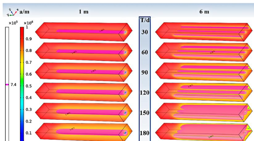
Figure 7. Comparison of effective drainage area between 1 and 6 m drill hole spacing at different times.
