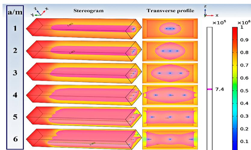
Figure 8. Gas pressure evolution and effective drainage area distribution under different drill hole spacings.
