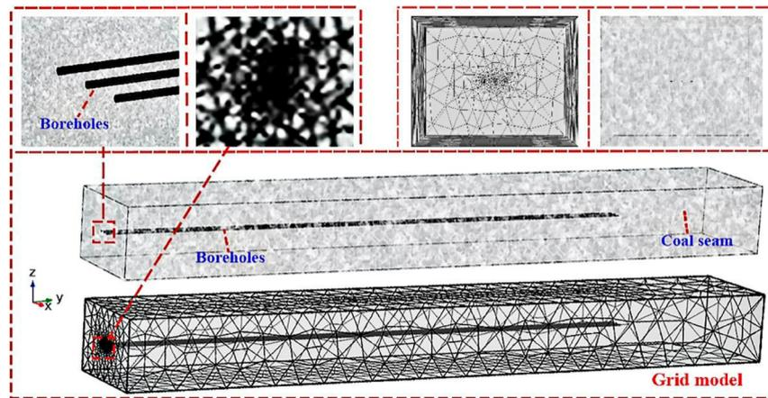
**Figure 1.** 3D model of coal seam gas predrainage.
