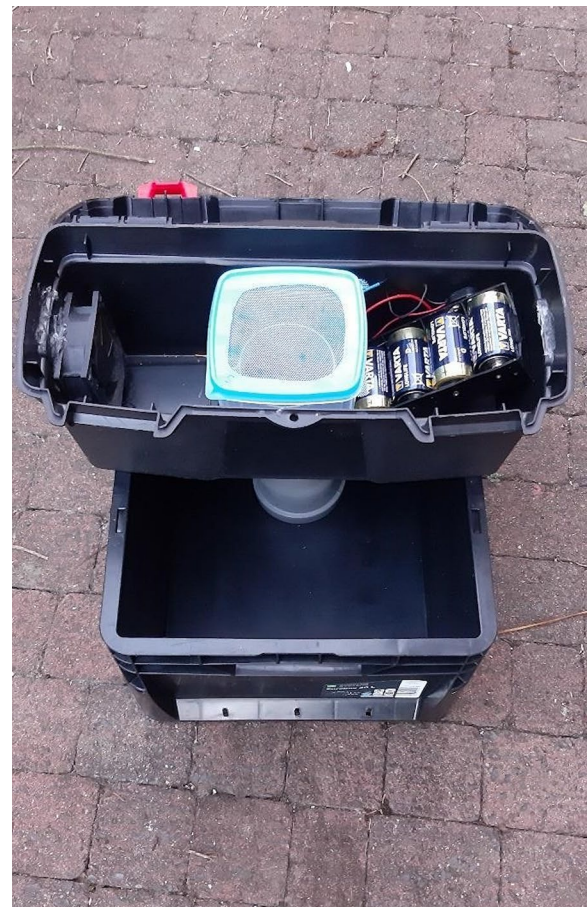
Fig. 1 Modified Reiter/Cummings type box gravid traps with honey-baited FTA cards
