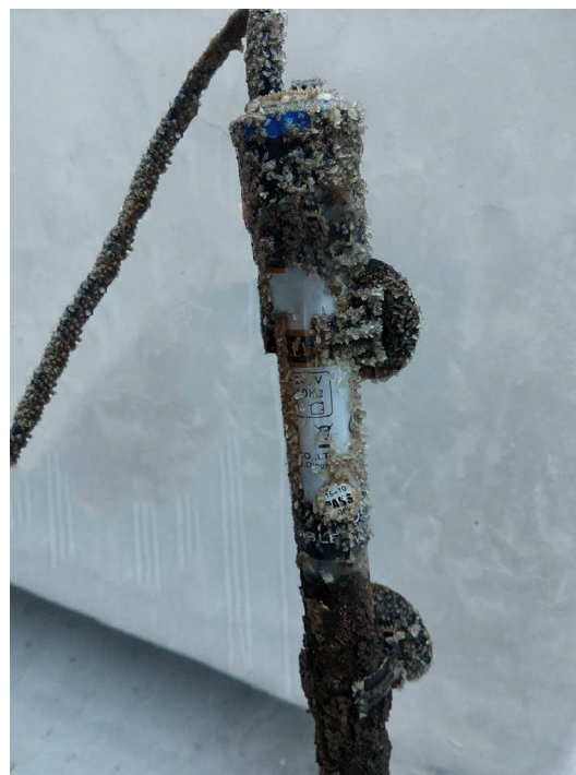
FIGURE 5 The inorganic salt crystallized on the heating rod in TK1 on day 57 (27 January 2016)
