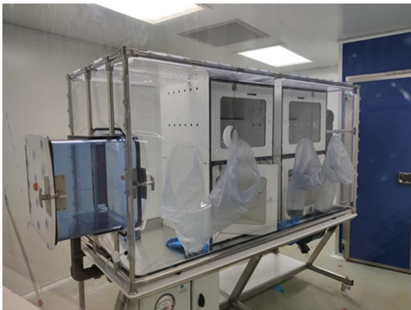
Fig. 1 BioFlex® B90 Flexible Film Trolley Isolator with HEPA filters containing pairs inside cages measuring 124.8 \times 51.6 \times 60 cm used in this experiment
