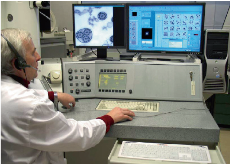
Fig. 14.5. The “server site” operator can flexibly control the EM alternatively by the software button controls and/or conventionally use the microscope panel knobset. The software supports a two-monitor image display; note the left screen showing the live image (abnormal cilia), the large right-hand screen displays the control panels (EM parameters, CCD camera, FFT-Image-Aid, and histogram), the images in the live computer memory, and the currently used database. The telepresence “feeling” in a telepathological consultation can be markedly increased by hooking it up to a parallel standard phone connection (a headset is a helpful tool enabling – here the author – freehand EM operation)
