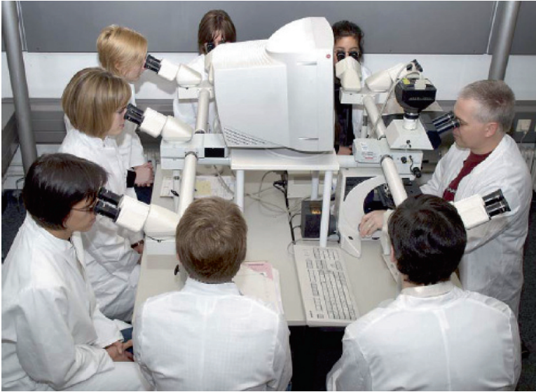
Fig. 14.1. Traditional local and simultaneous image sharing at a multiheaded light microscope during the intradepartmental daily case discussion. Every observer can see exactly the same tissue image area at the magnification chosen by the case-referring pathologist and make comments on the rendered diagnosis. (Courtesy of Pathology Department University Hospital/Regensburg)
