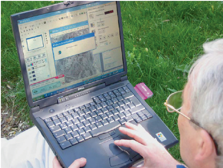
Fig. 14.9. Demonstration of an outdoor wireless remote access on the telepathology system in Regensburg. The “client” expert notebook was equipped with a dedicated UMTS PCMCIA-card ( pink colored ), which uses the new telecommunication channel of T-Mobile and Vodafone company. We experienced stable connections, but the available bandwidth (0.320 Mbps) caused a significant image transfer delay. (UMTS-cards, courtesy of T-Mobile and Vodafone Regensburg)
