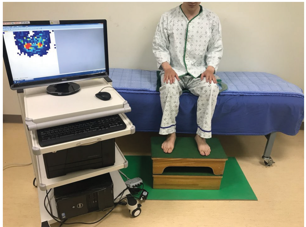
Fig. 1. Posture for measuring the sitting pressure. After sitting on the force platform, the patient places both feet on the ground, both hands on their lap, and sits upright without support for approximately 10 seconds, at the end of which, the pressure exerted by the patient's buttocks is measured.
