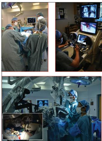
**Figure 3: Top left: Surgeon's posture in conventional surgery, top right: Surgeon at the robot workstation, bottom: NeuroArm robot operating in conjunction with the surgical assistant in the operating room; inset: NeuroArm tools within the surgical corridor**
