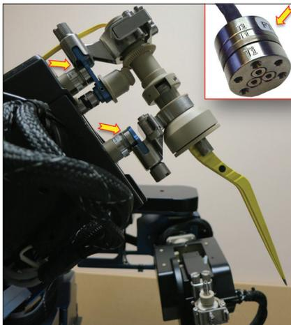
Figure 6: Titanium Nano 17 force sensor used in neuroArm (arrows)
