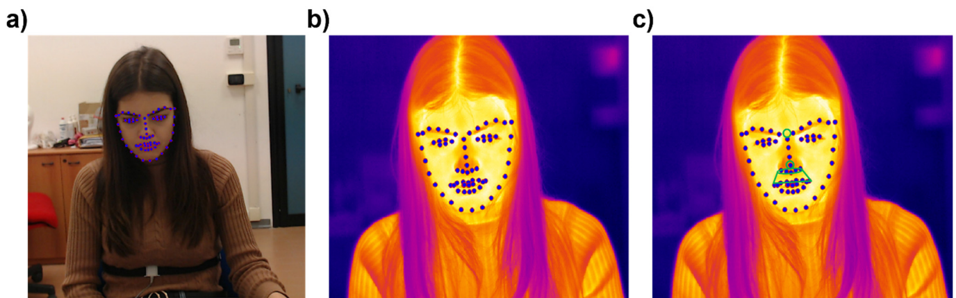
Figure 3. Thermal tracking pipeline. (a) Facial landmarks' automatic recognition in the visible domain. (b) Facial landmarks' identification on the corresponding IR images. (c) ROI identification with respect to the facial landmark. The green circles correspond to the four facial regions tracked, which are: the nose tip, nostrils, perioral, and corrugator area.
