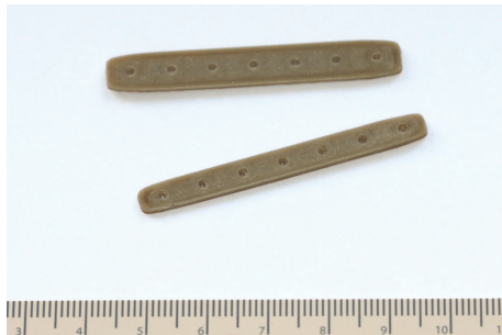
FIGURE 4: 3D printed PEEK osteosynthesis plates. Thieringer FM et al. AMPA 2017.
