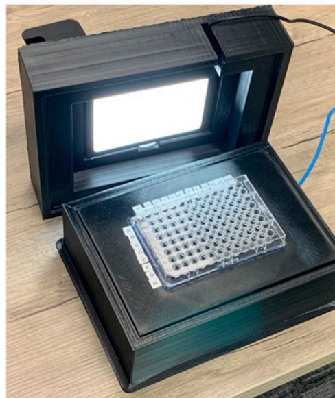
(B) Plate reader with top removed
