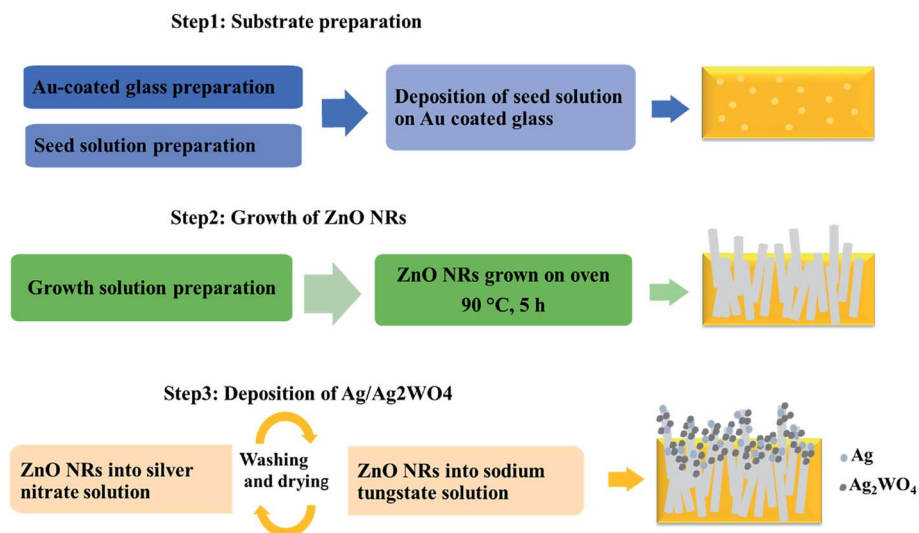
Fig. 1 Schematic diagram of preparation of ZnO NRs and the \text{ZnO}/\text{Ag}/\text{Ag}_2\text{WO}_4 photoelectrodes.
