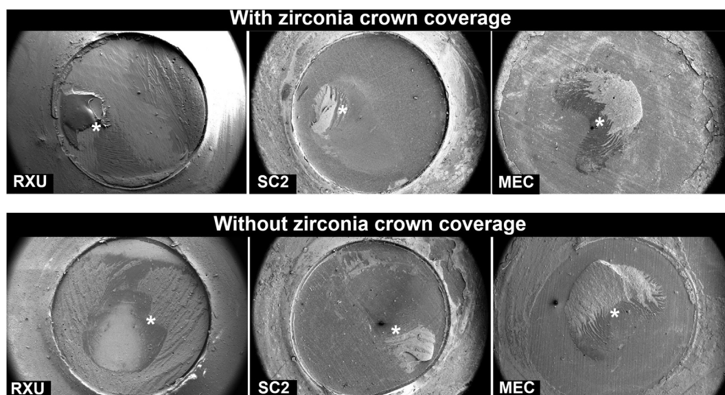
Figure 3 Representative SEM images of the fractured zirconia specimens with (top) and without (bottom) zirconia crown coverage. Asterisks indicate the junction between the resin cement and zirconia. Varying degrees of mixed failure pattern of adhesive failure at the interface between zirconia and resin cements, and cohesive failure within resin cement were observed in all examined surfaces.
