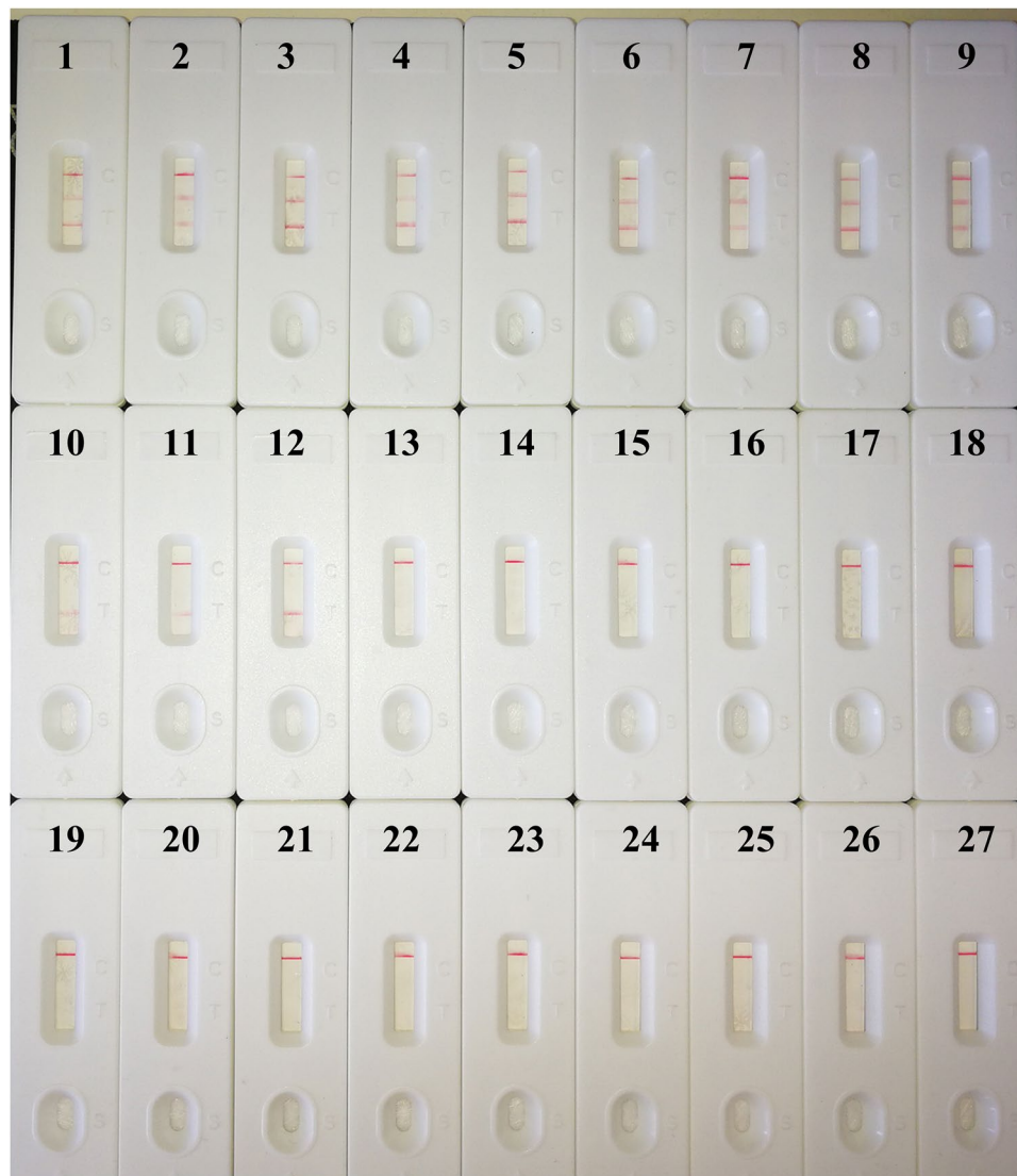
Figure 5. Specificity of duplex MCDA-LFB assay using different bacterial strains. The m-MCDA amplifications were carried out using different genomic DNA templates and the results were indicated using LFB. Biosensors 1–9, A. baumannii strains with bla OXA-23-like gene; Biosensors 10–12, A. baumannii strains without bla OXA-23-like gene; biosensors 13–27, Listeria monocytogenes , Bacillus cereus , Citrobacter braakii , Citrobacter freundii , Corynebacterium ammoniagenes , Escherichia coli , Klebsiella pneumoniae , Proteus mirabilis , Providencia rettgeri , Pseudomonas aeruginosa , Serratia marcescens , Serratia marcescens , Staphylococcus aureus , Staphylococcus epidermidis , Streptococcus salivarius .
