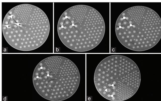
**Figure 4:** Cross section of Jaszack phantom without activity showing streak artifacts due to iodine water interface contrast in computed tomography acquisition with (a) no filter (b) Cu 1 mm (c) Cu 2 mm (d) Cu 3 mm (e) Cu 4 mm filter while computed tomography acquisition
