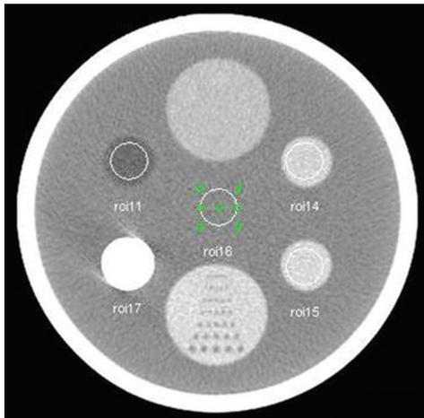
Figure 9: Cross section of Philips computed tomography quality control phantom
