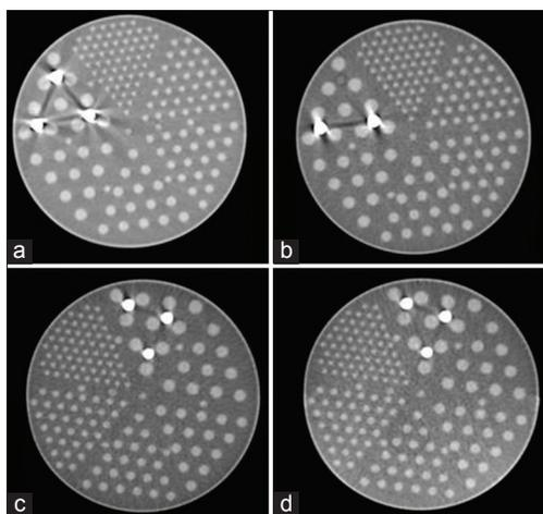
Figure 6: Cross section of Jaszack phantom without activity showing streak artifacts due to iodine water interface contrast in computed tomography acquisition with (a) no filter (b) Cu 2 mm + Al 1 mm (Cu2Al1) (c) Cu 2 mm + Al 2 mm (Cu2Al2) (d) Cu 2 mm + Al 3 mm (Cu2Al3) while computed tomography acquisition
