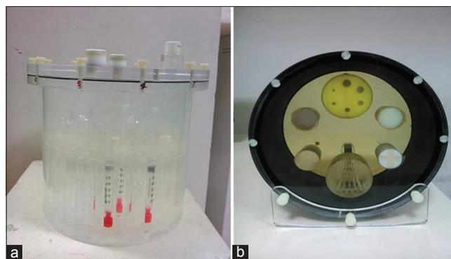
Figure 1: (a) Jaszack phantom with iodine contrast filled syringes (b) Philips computed tomography quality control phantom having six different density inserts of polyethylene, teflon, perspex (acrylic), lexan, nylon (aculon), and water
