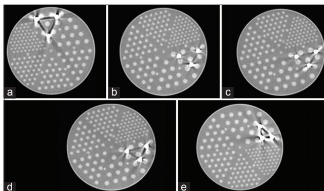
**Figure 3:** Cross section of Jaszack phantom without activity showing streak artifacts due to iodine water interface contrast in computed tomography acquisition with (a) no filter (b) Al 1 mm (c) Al 2 mm (d) Al 3 mm (e) Al 4 mm filter while computed tomography acquisition
