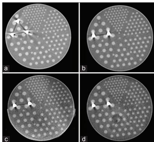
**Figure 5:** Cross section of Jaszack phantom without activity showing streak artifacts due to iodine water interface contrast in computed tomography acquisition with (a) no filter (b) Cu 1 mm + Al 1 mm (Cu1Al1) (c) Cu 1 mm + Al 2 mm (Cu1Al2) (d) Cu 1 mm + Al 3 mm (Cu1Al3) while computed tomography acquisition
