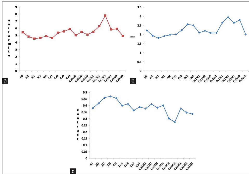
Figure 10: Variation of (a) uniformity (b) root mean square (c) contrast for cold sphere, of single photon emission computed tomography/computed tomography images of Jaszack phantom corrected with X-ray beam using different filter thickness and filter combinations
