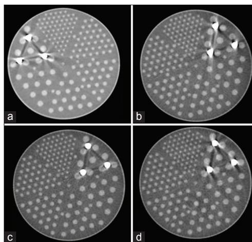
Figure 7: Cross section of Jaszack phantom without activity showing streak artifacts due to iodine water interface contrast in computed tomography acquisition with (a) no filter (b) Cu 3 mm + Al 1 mm (Cu3Al1) (c) Cu 3 mm + Al 2 mm (Cu3Al2) (d) Cu 3 mm + Al 3 mm (Cu3Al3) while computed tomography acquisition
