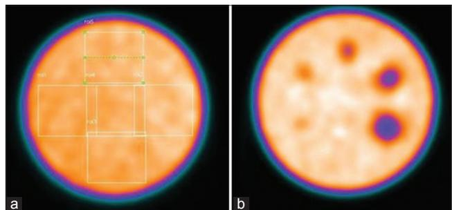
**Figure 2: Cross section of Jaszack phantom (a) of uniform slice showing regions of interest's placed at five different positions for calculation of average counts (b) showing cold spheres**
