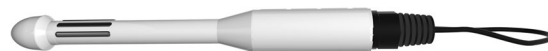
Figure 2. The model of the prototype enabling tetrapolar electrode configuration and comprised with a single set of 4 electrodes.
