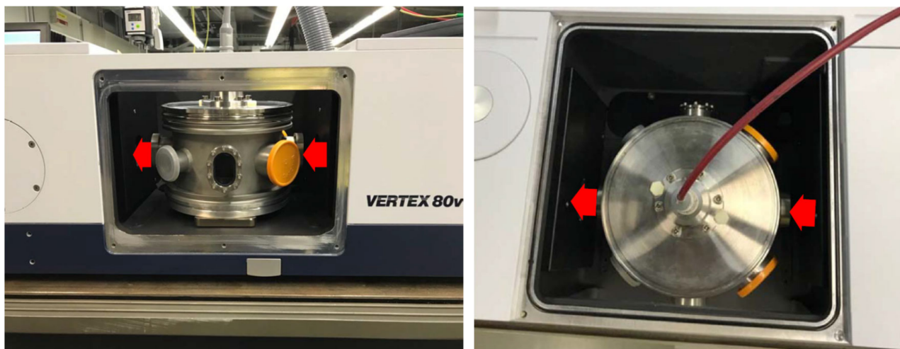
Figure 7. Side and top view photographs of the plasma reactor (see also Figure 4a) inside the sample compartment of the FTIR spectrometer, for in situ single-pass absorption measurements. The infrared passage through KBr windows is marked by the red arrows. The Faraday cage design of the reactor and its coaxial power supply cable protects against any possible electromagnetic perturbation to the FTIR instrument.
