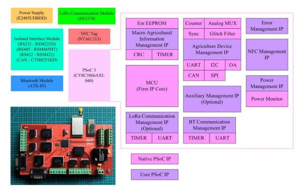
Figure 5. Hardware structure of in-field service node.
