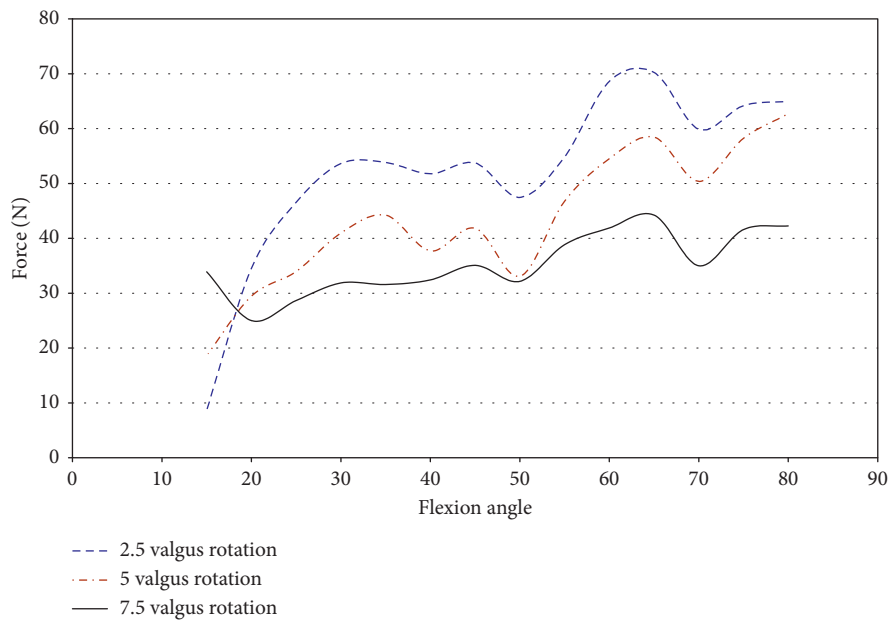
FIGURE 24: Magnitude of force measured by JR3 UFS vs flexion angle; valgus rotation 50067.
