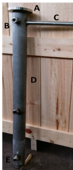
Figure 3. Fluidization reaction reactor: (A) top section of reactor, (B) gas sampling tube, (C) supporting beam, (D) reactor body, and (E) fluidized gas input tube.
