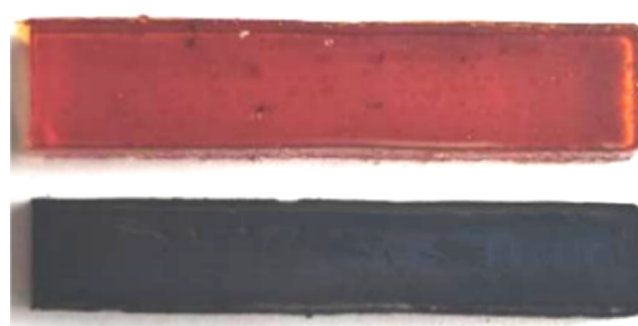
Figure 10. Images of the cured ALSZ(10:1)-1%cumenyl-0.5% CoCPA casting body (top image) and its pyrolytic ceramic monolith after pyrolysis at 800 °C (bottom image).
