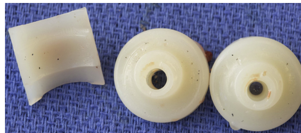
Figure 3 Polyethylene wear, pitting, and metal particle embedding of an explanted Nexel TEA. Note that the titanium particles are located in the portions of the polyethylene that articulates with the titanium surfaces of the ulnar component. TEA, total elbow arthroplasty.
