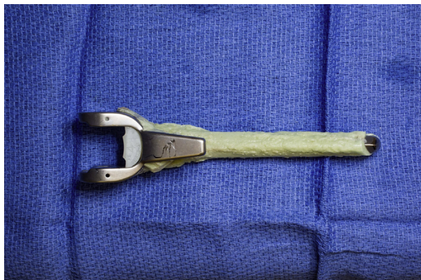
Figure 2 Explanted Nexel TEA demonstrating failure at the bone-cement interface. TEA, total elbow arthroplasty.
