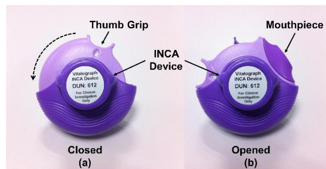
FIGURE 2. To open a closed Diskus™ DPI (a) slide thumb grip in direction of dashed arrow until mouthpiece is fully exposed as seen in (b). INCA™ device attaches onto Diskus™ inhaler to record audio signal of inhaler use.
