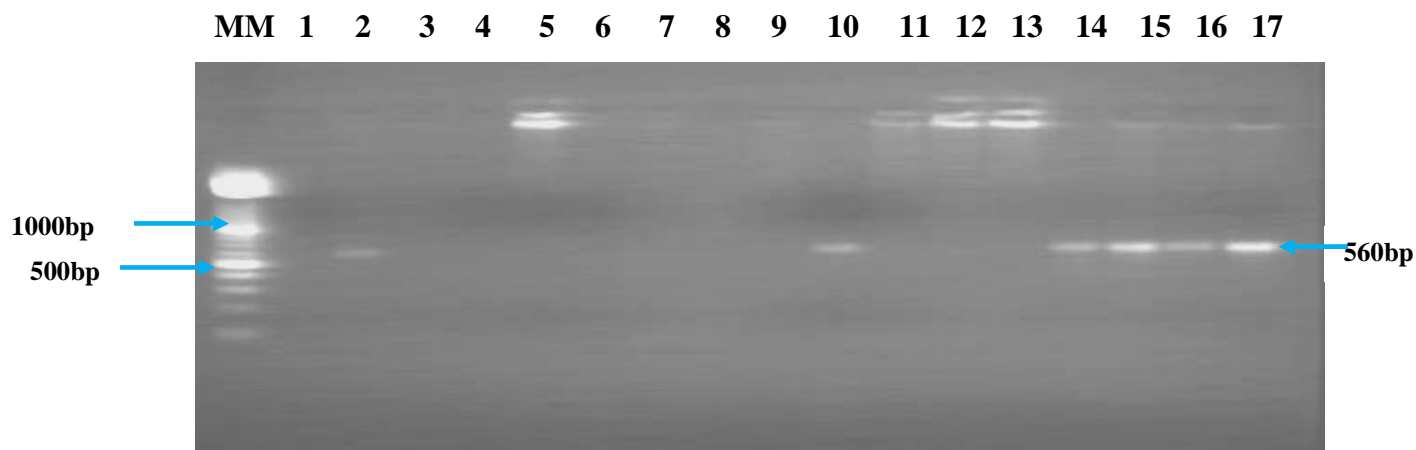
Figure 1: Representative gel showing nested PCR products on 1.5% agarose gel electrophoresis of P. falciparum negative blood filters determined by microscopy. MM is the molecular weight marker, Lane 1, represents the negative control, Lane 2, the positive control and lanes 3-17 are the P. falciparum negative samples by microscopy from the epidemic areas.
