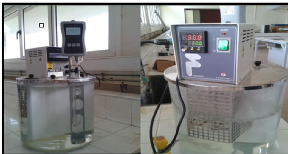
Figure 19. Picture of Cannon–Ubbelohde viscometer for viscosity measurements.
