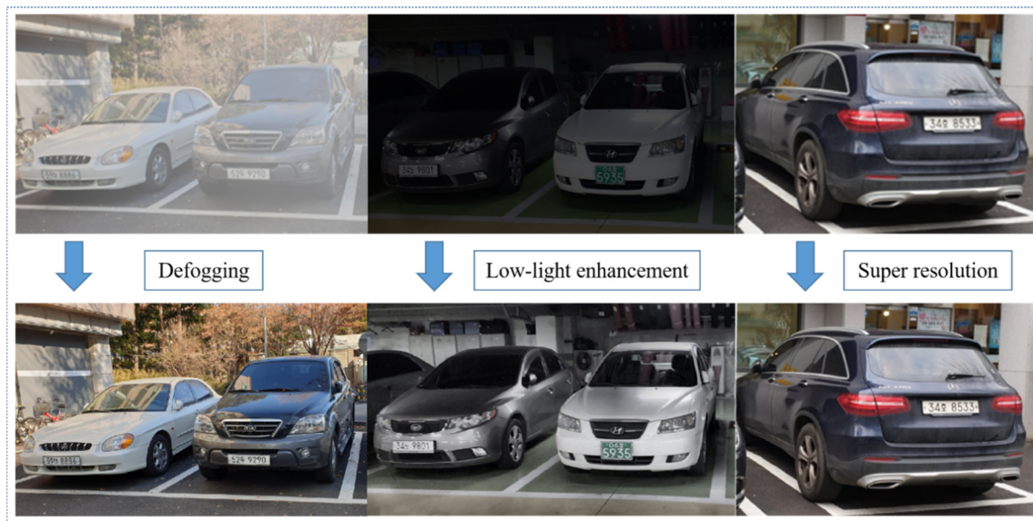
Figure 6. The visual effect of three image preprocessing technologies, which include defogging, low-light enhancement, and super-resolution.
