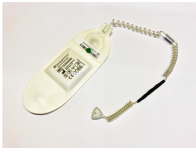
Figure 1 The SensiumVitals patch. The SensiumVitals patch is attached to the patient's chest and monitors heart rate and respiratory rate. The black 'wire' sensor is the external axillary temperature monitoring device.
