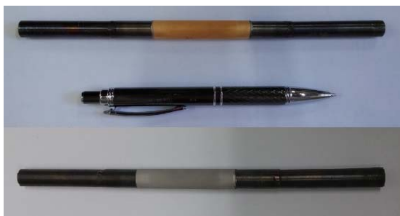
Figure 7. Picture of the supported Pd-Au membrane before tests (top) and after (bottom).
