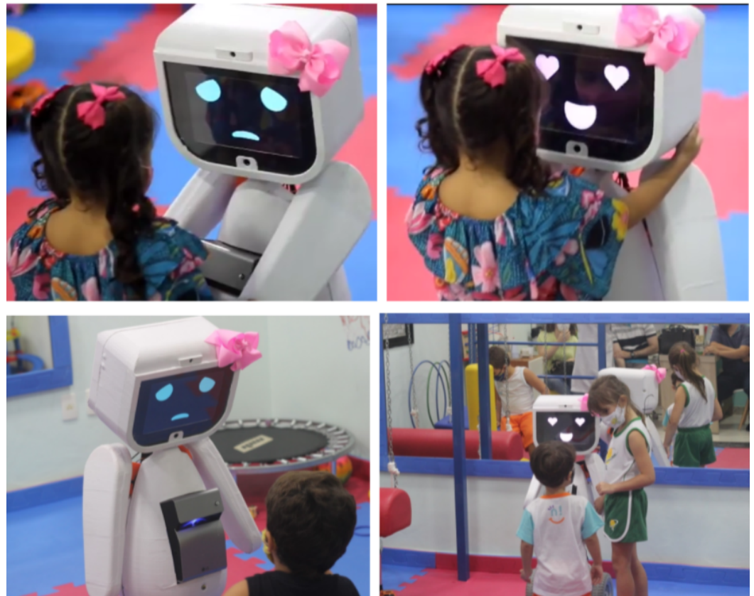
Figure 1. MARIA T21 interacting with children with ASD and DS, and demonstrating its ability to express emotions in the face.
