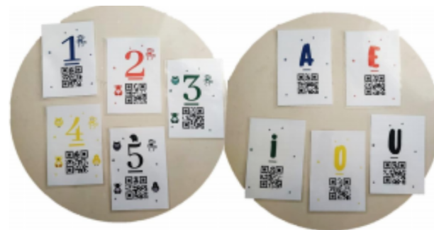
Figure 10. Cards approximately 14 cm long containing QR codes that children must show to the robot. The camera on the robot’s head detects if the card is correct based on the QR code.
