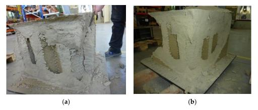
**Figure 24.** Side views of the specimen after the test: (**a**) before and (**b**) after the removal of the material isolated (only in part) by the sliding surfaces.
