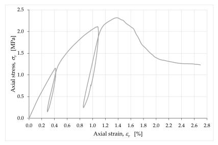
**Figure 26.** Complete average curve of the axial stress with respect to the axial strain, obtained from the acquisitions of the LVDTs placed between the corners of the metal plates for the distribution of the load.
