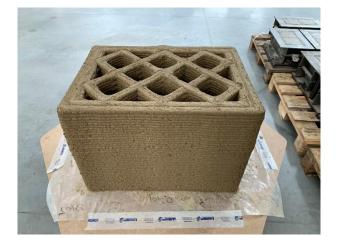
Figure 5. 3D-printed specimen in the fresh state.
