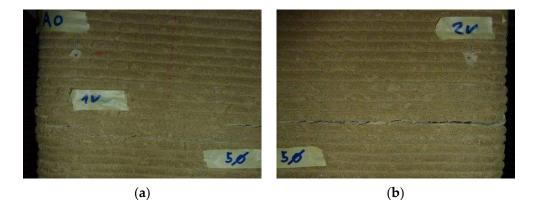
**Figure 11.** Details of the detachments between the horizontal layers of the side to the left of the operator: (a) left detachment, which reaches edge 1; (b) right detachment, which reaches edge 2.
