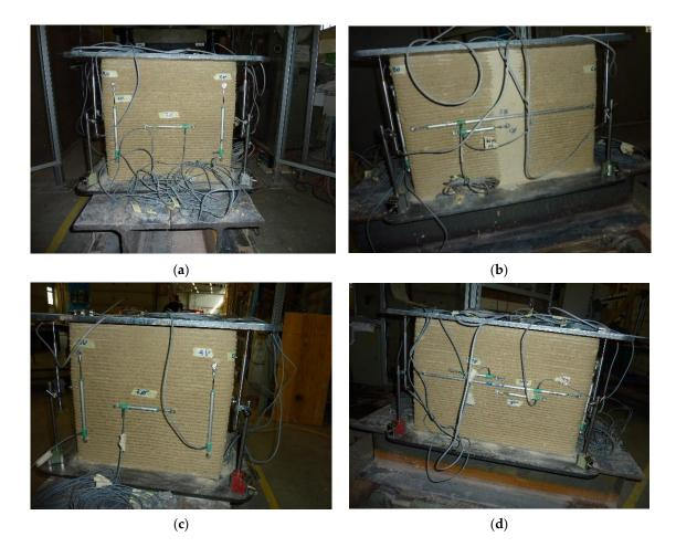
**Figure 8.** Side views of the LVDTs, listed from left to right: (a) LVDT VA, LVDT V1, LVDT H5, LVDT V2, LVDT VB on the short side face to the left of the operator; (b) LVDT VB, LVDT H9, LVDT H6, LVDT VC on the long side face in front of the operator; (c) LVDT VC, LVDT V3, LVDT H7, LVDT V4, LVDT VD on the short side face to the right of the operator; (d) LVDT VD, LVDT H10, LVDT H11, LVDT H8, LVDT VA on the long side face on the opposite side of the operator.
