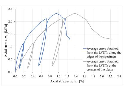
**Figure 14.** Average curves of the axial stress with respect to the axial strains  $\varepsilon_e$  and  $\varepsilon_c$ .
