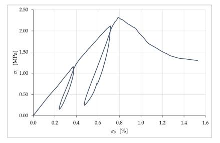
**Figure 21.** Curve of the axial stress,  $\sigma_v$ , with respect to  $\varepsilon_{\vartheta}$  (apparent volumetric strain).
