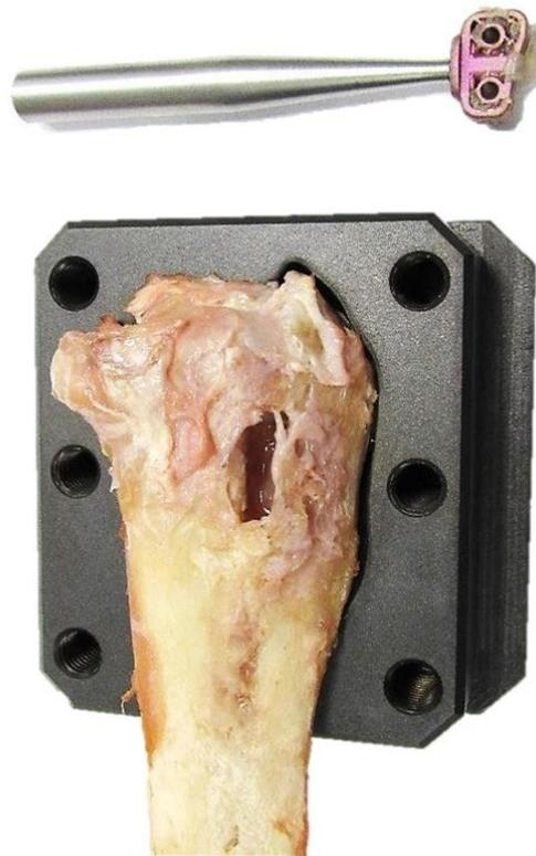
**Figure 8.** A torn TTA CF implant after biomechanical testing.
