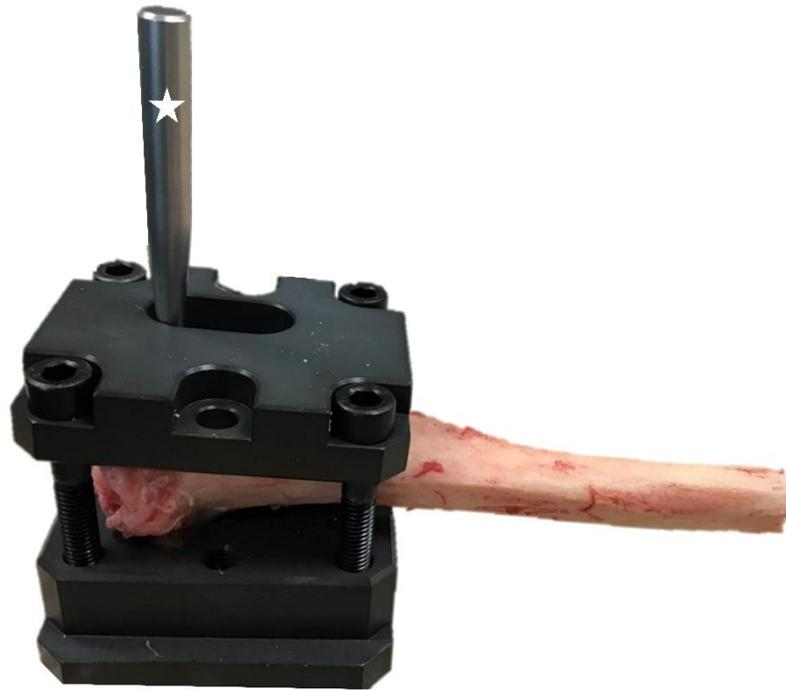
**Figure 6.** Specimen prepared for mechanical testing. A screwed custom bar is marked with an asterisk.
