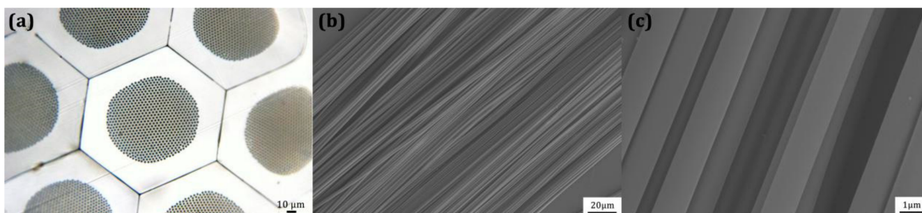
Figure 8. (a) Cross-sectional image of the 3rd-draw PS/PMMA fiber, (b) SEM image of PMMA microwires with the diameter of about 1.6 \mu\text{m} after dissolving outer PS of the 3rd-draw PS/PMMA fiber, (c) enlarged SEM image of PMMA microwires.
