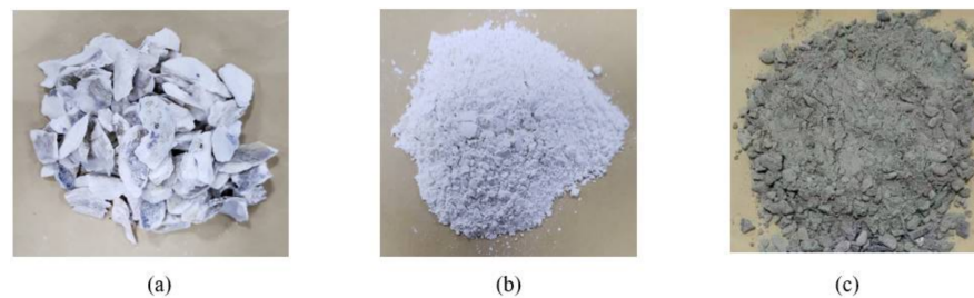
Figure 1. Materials: (a) NCOS (10–13 mm); (b) COSP; (c) MWR ( \leq 5 mm).
