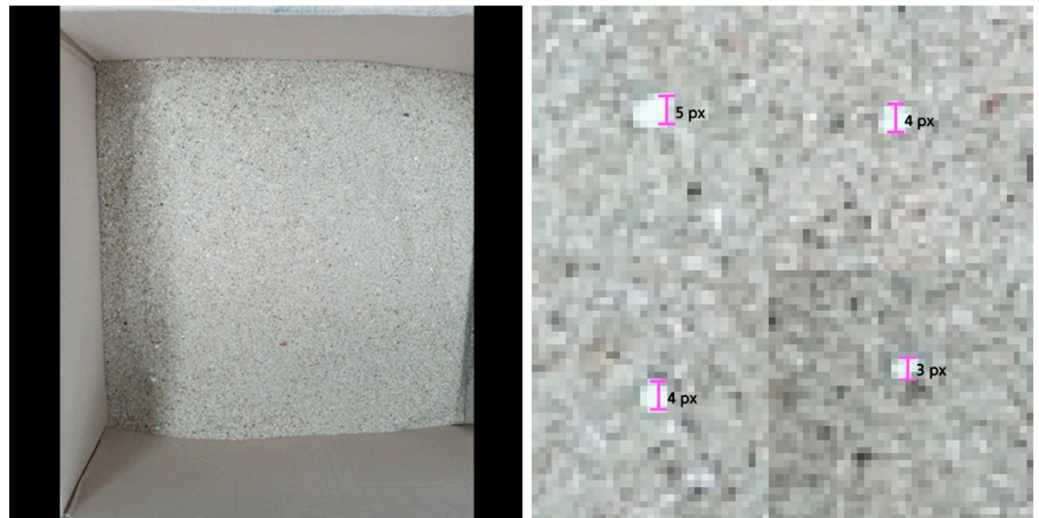
Figure 7. Original sand photo and a photo to show the size of microplastics.
