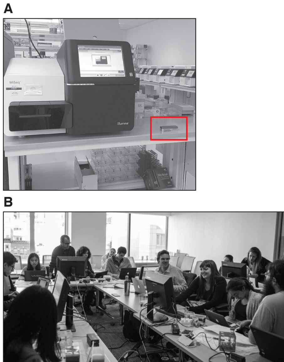
Figure 1. The Ubiquitous Genomics class. (A) Illumina MiSeq benchtop sequencer (left) and the MinION sequencer made by Oxford Nanopore Technologies (right; red rectangle). (B) The class during a hackathon. DOI: 10.7554/eLife.14258.002
