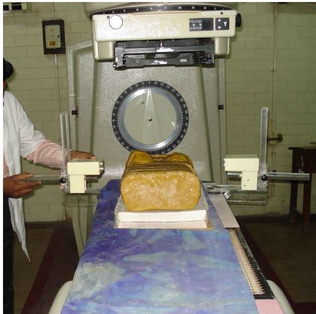
FIG. 2. Photograph of the UPMMD sensor device experimental setup in radiotherapy machine.
