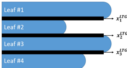
FIG. 2. Simple example of beam’s eye view for the left leaf bank, showing the location for tongue and groove fluence calculation. The dark strips between adjacent leaves represents the 1 mm area for fluence calculation.
