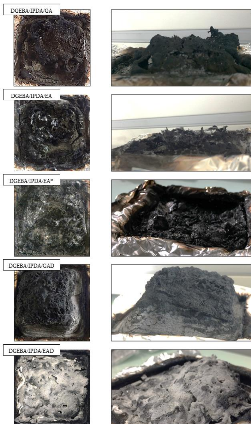
Figure 15. Cone calorimeter residues of the prepared thermosets.
