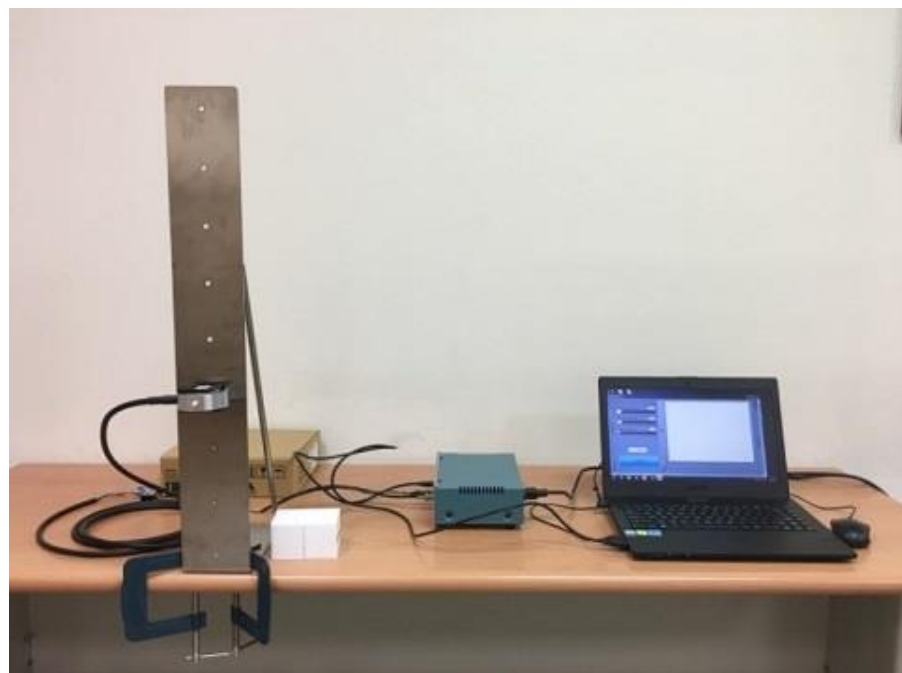
Figure 2. The setting of equipment for the measure of press strength.
