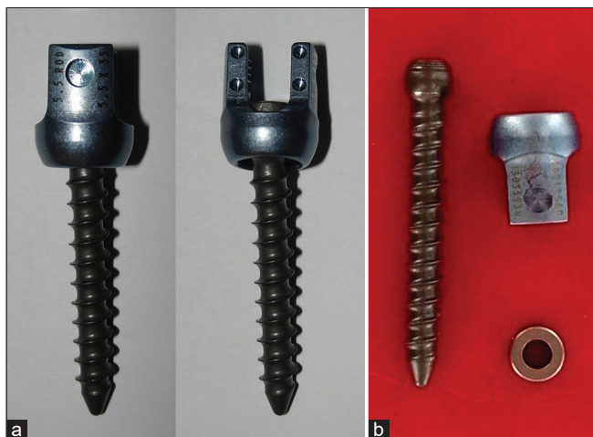
Figure 2: Polyaxial pedicle screws before use. These multiaxial screws have 360° head polar mobility (a). Picture of the dislocated polyaxial screw: The screw head was detached from screw shank (b).
