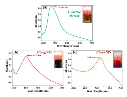
Figure 4. Absorption spectra of (a) extract of C. inerme leaves, (b) CI-Au NPs and (c) CI-Ag NPs.
