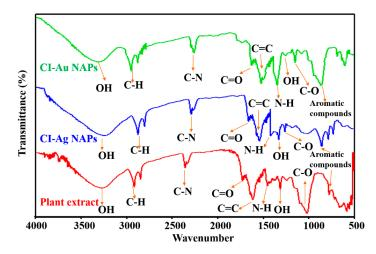
Figure 5. FT-IR spectra of green synthesized CI-Au NPs, CI-Ag NPs, and the C. inerme leaves extract.
