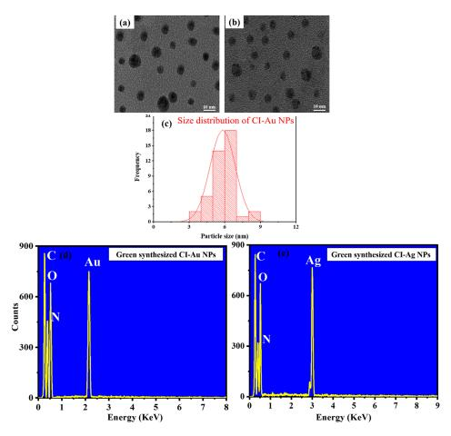
**Figure 3.** (**a**,**b**) TEM, (**c**) DLS, and (**d**,**e**) EDX spectra of green synthesized CI-Au and CI-Ag NPs, respectively, using leaves extract of *C. inerme*.
