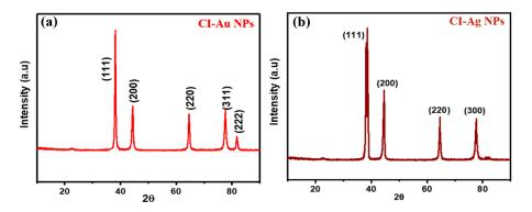
**Figure 2.** XRD patterns of green synthesized (**a**) CI-Au NPs and (**b**) CI-Ag NPs using leaves extract of *C. inerme*.
