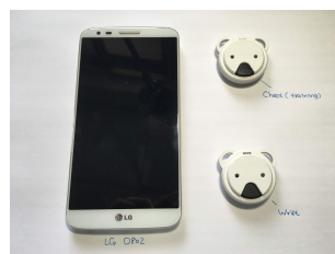
Figure 9. Required hardware in the sleep posture monitoring system. On the left is an Android smartphone, on the right are two wearable sensors.
