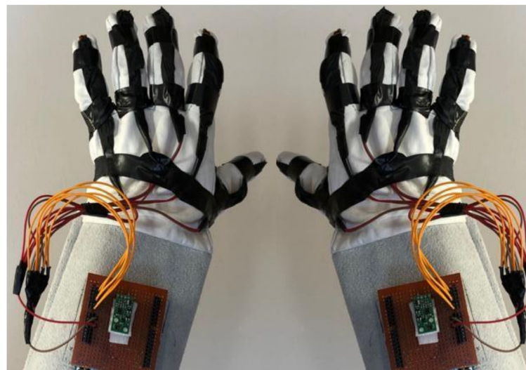
Figure 4. A pair of smart glove designs built with Flex and IMU sensors and an STM32 card.
