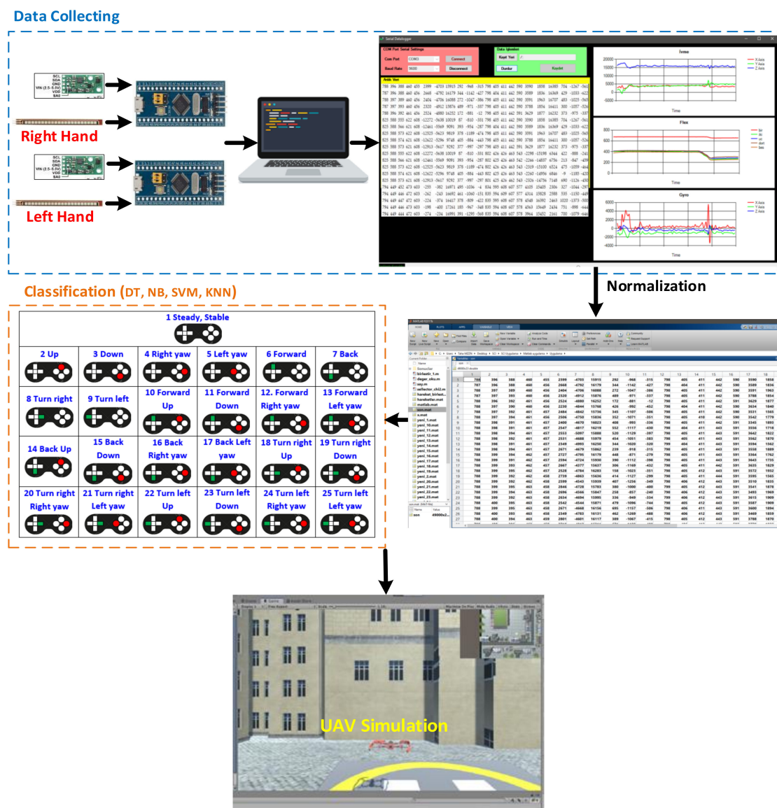
Figure 6. The stages of classifying hand gestures via a pair of smart gloves that can be used in real time with the help of machine learning algorithms and controlling the UAV in a simulation environment.
