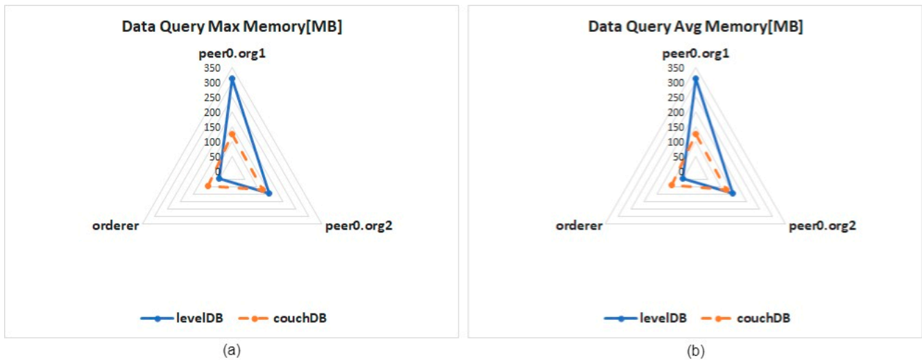
Figure 14. Memory usage for single data query: (a) maximum memory usage, (b) average memory usage.
