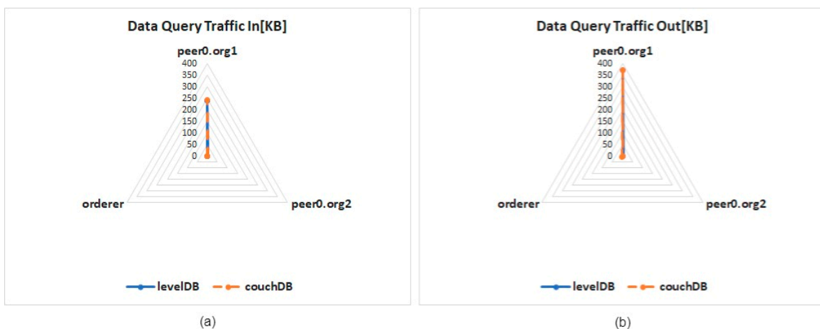
Figure 15. Network traffic for a single data query: (a) incoming packets, (b) outgoing packets.
