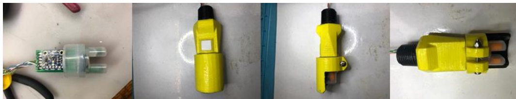
Figure 9. Encasing and waterproofing the turbidity sensor.
