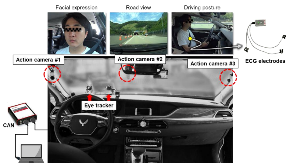
Figure 1. Driver cockpit for the on-road evaluation of passive task-related fatigue of the driver.
