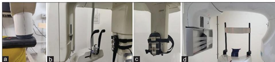
Figure 2: Pictorial representation of air kerma measurement towards diagnostic reference levels assessment used for intraoral (a), panoramic (b), cephalometric (c), and cone beam computed tomography (d) radiography
