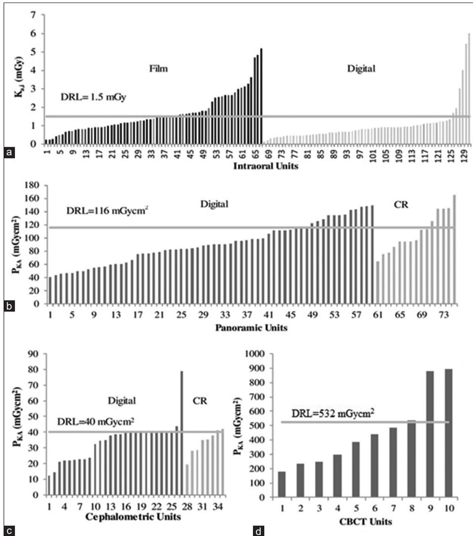
**Figure 3:** Proposed diagnostic reference levels (horizontal bar) for intraoral (a), panoramic (b), cephalometric (c) and cone beam computed tomography (d) examinations
